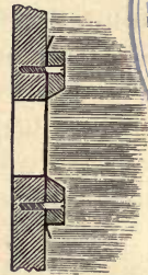
Fig. 79.—Section of Parchment Diaphragm.
